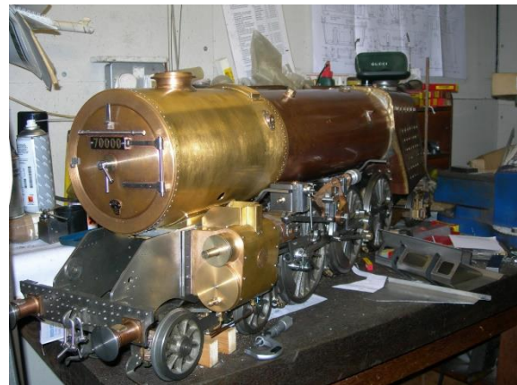
Boiler without Cladding
