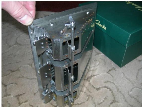
Ashpan showing Dampers
